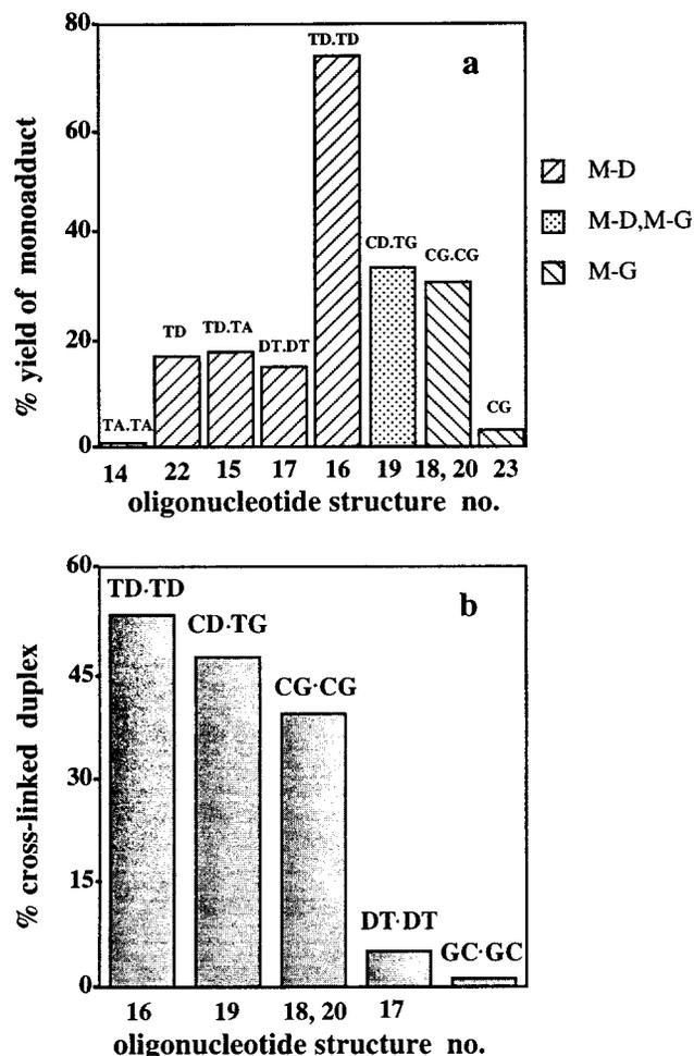
**Figure 4.** Yields of monoalkylation and bifunctional alkylation (cross-linking) of DAP or guanine by MC in oligonucleotides: (a) monoadduct M-D (**10a**) or M-G (**6a**) and (b) cross-linked duplex oligonucleotides. The dinucleotide sequences above the bars correspond to the alkylated or cross-linked sites of the oligonucleotides. Average deviation from the mean value of three experiments never exceeded  $\pm 15\%$  in the cases when it was determined.
